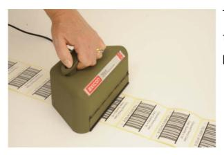
The Axicon 7025-S being used – again the verifier is in contact with the barcode.
