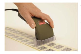
The Axicon 6025-S - Note that all four corners of the verifier are touching the label - it is neither being "rocked" forwards or backwards.
