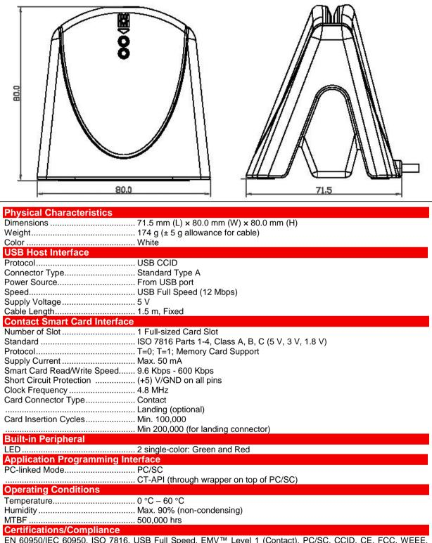
EN 60950/IEC 60950, ISO 7816, USB Full Speed, EMV™ Level 1 (Contact), PC/SC, CCID, CE, FCC, WEEE, RoHS, REACH, TAA (USA), J-LIS (Japan), VCCI (Japan), PBOC (China), Microsoft® WHQL
