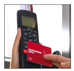
As smart card technology becomes more widely accepted in the market, developers find an opportunity to offer better usage experience and security by adding more features to smart card reading devices. The ACR89U-A2 Handheld Smart Card Reader with NFC tag support is primarily designed for multiapplication that can access any contact and contactless smart cards following the ISO 7816 and ISO 14443 standards.
