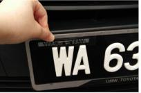
\*\* Please DO NOT place the sticker on metal surface / windscreen or near any metallic object. Metal will severely inhibit reading range.
