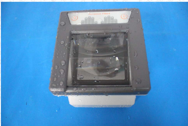
Photo 5 After IPX4 test
