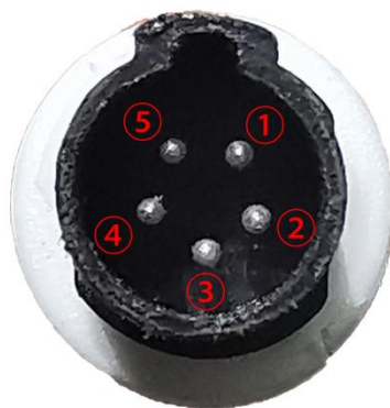
Figure 5.1.2 UR1A GPIO terminal location
