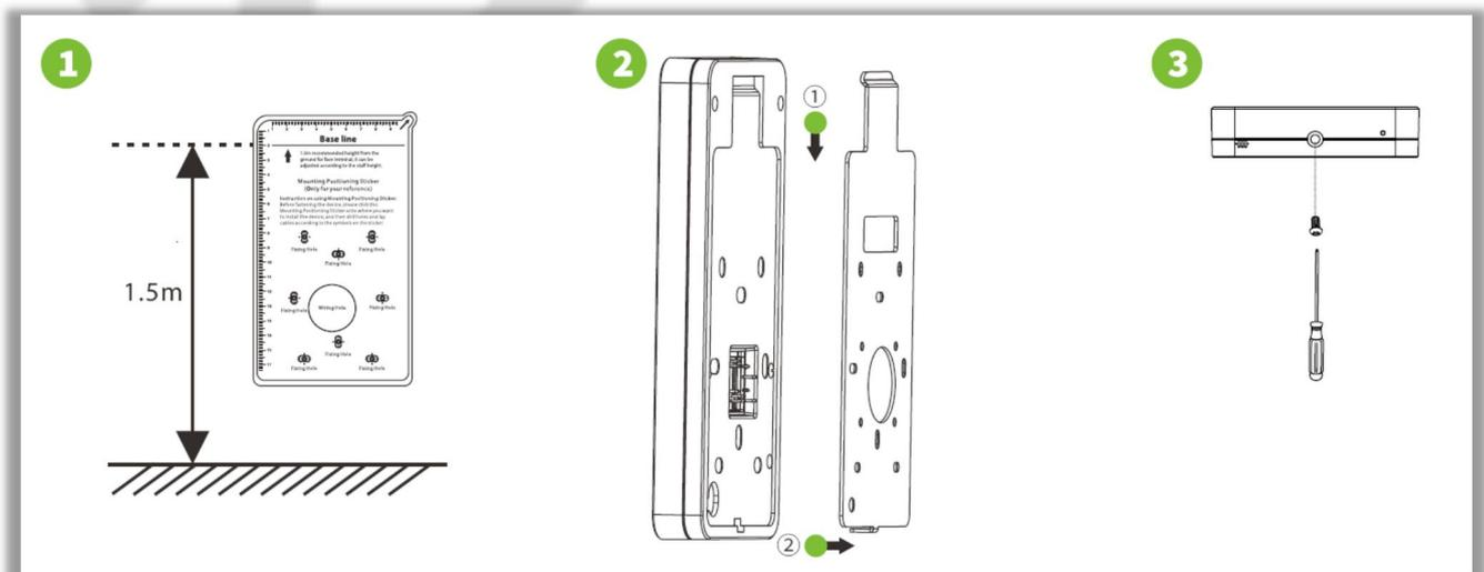
Step 1: Attach the mounting template sticker to the wall, and drill holes according to the mounting paper. Fix the back plate on the wall using wall mounting screws.
