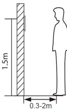
The distance between the device and a user whose height is within 1.4m-1.8m is recommended to be 0.3-2m. Users may slightly move forwards and backwards to improve the quality of facial images captured.
