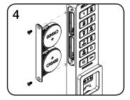
Re-Insert the battery pack and screw cover plate in place.
