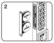
Pull the battery pack from the front housing.
