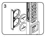
Remove batteries and replace with two premium lithium CR2450 batteries.
