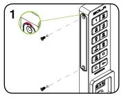
Remove the 2 battery cover plate screws.
