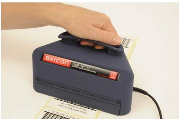
The Axicon 7015 being used - again the verifier is in contact with the barcode.
