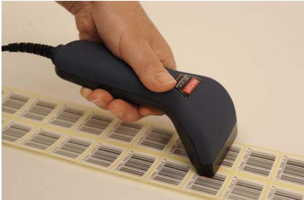
The Axicon 6015 - Note that all four corners of the verifier are touching the label - it is neither being "rocked" forwards or backwards.
