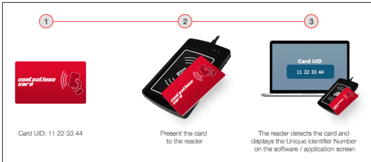
Figure 1: ACR1281U-C2 Sample Application
